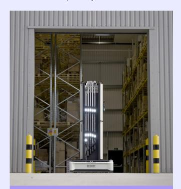
A fully autonomous robot can detect its environment, make decisions based on what it perceives and/or has been programmed to recognise, and then act without human intervention.
