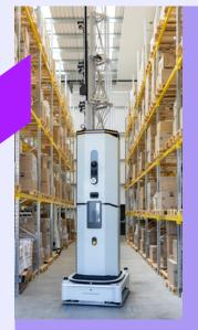
The platform automates data collection and builds real-time digital twins that unlock insights across all levels of warehouse operations. Dexory's robots measure, count, track and find inventory across warehouses as they navigate the racks, without workflow disruption.
